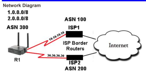
This configuration allows Router 1 (R1) to peer with BGP speakers in other autonomous systems. The **route-map localonly** command allows only the locally generated routes to be advertised to both of the ISPs. This prevents Internet routes from one ISP to the other ISP and prevents the risk that your AS becomes a transit AS for Internet traffic.
