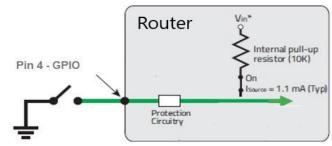
The voltage on Pin 4 when the high side pull-up is enabled (depends on the Vin and power consumption.
