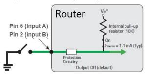
Maximum current the voltage output can provide (depends on Vin)
