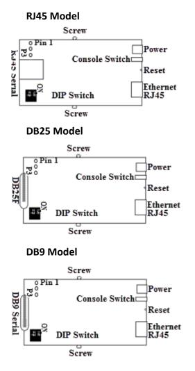
3. To change the Power Pin out, locate P3. For the fixed 5V DC output, jumper pins 1 and 2. For the output to equal the external adapter input, jumper pins 2 and 3.
