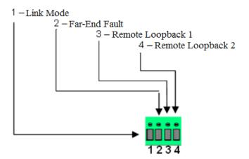
**Note:** All switch changes take effect immediately and will result in a link reset on both fiber ports.
