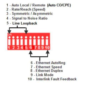
NOTE: All switch changes take effect immediately and will result in a link reset on both the Line and the Ethernet ports.
