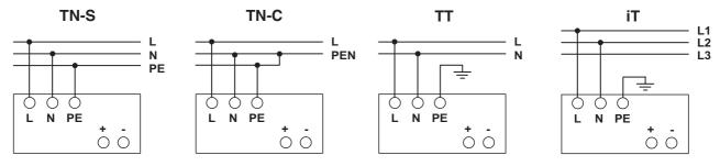
The 100 V AC ... 240 V AC connection is made using the L, N and PE screw connections.
