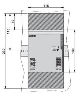
Mounting position: Installation depth 152.5 mm (+ DIN rail)
