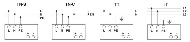
The 100 V AC ... 240 V AC connection is made using the L, N and PE screw connections. The device can be connected to 1-phase AC systems or to two of the phase conductors of three-phase networks (TN, TT or iT system in acc. with VDE 0100-300/IEC 60364-3) with nominal voltages of 100 V AC ... 240 V AC. The device also continues to work on short-term input voltages > 300 V AC.
