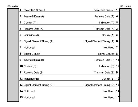
Figure 3 - 15 V.11/X.21 Null-Modem Cable
