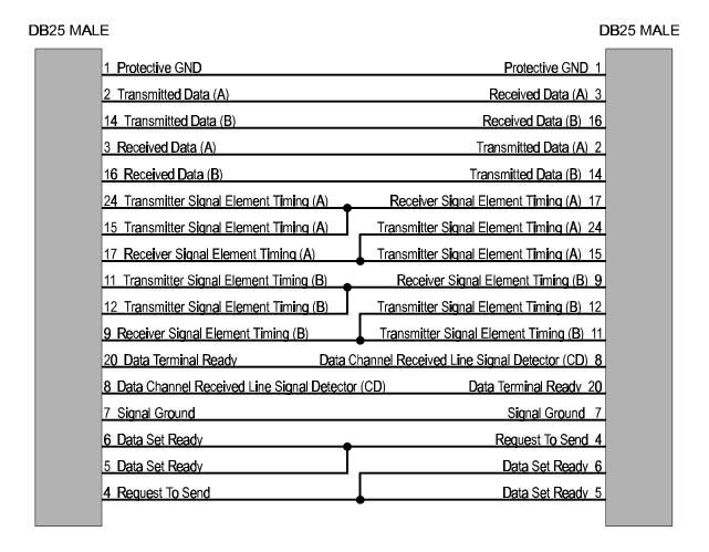
Figure 3 - 11 V.35 Null-Modem Cable
