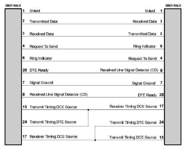
Figure 3 - 8 RS232 Null-Modem Cable
