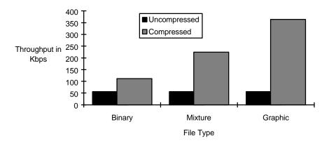
Figure 1 - 6 Typical Throughput Over 56 Kbps Link
