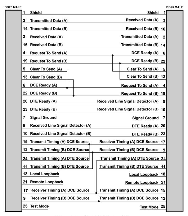
Figure 3 - 13 RS530 Null-Modem Cable
