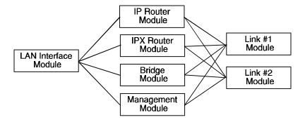
Figure 1 - 1 IOLINK-CENTRAL Ethernet Bridge/Router Block Diagram
