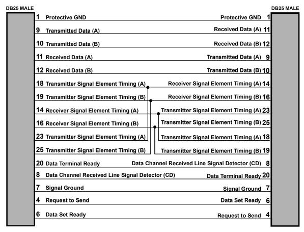
Figure 3 - 12b Early model V.35 Null-Modem Cable
