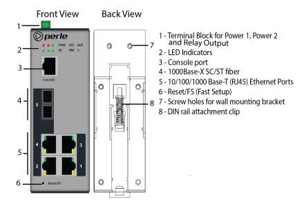
**Note:** Fiber Port may appear different, depending on the type of fiber port installed.
